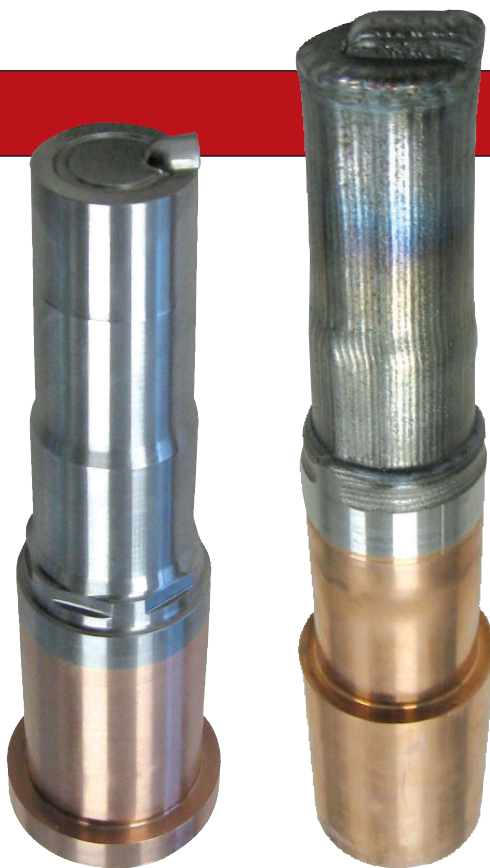
Steel-clad copper cores for high productivity tooling in aluminum die casting. The steel is bonded to copper through a proprietary buffer material. Image courtesy of DMD 3D.
