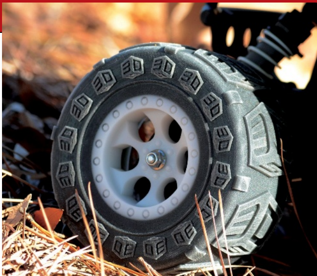
Sample tire for a remote-control toy car, with both black rubber-tire and rigid white wheel-sections built as a multi-material part on a 3D Systems Projet 5500. Image courtesy of 3D Systems.
